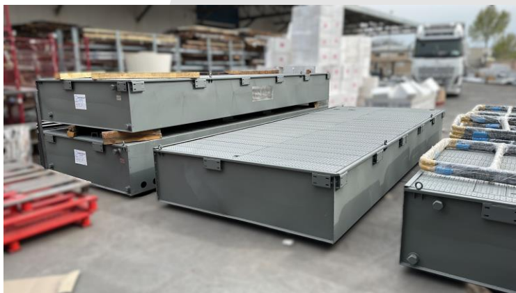
Anti-corrosion protection for steel retention tanks
