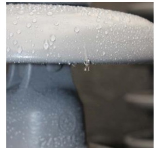
Hydrophobicity of the Midsun® HVIC coating
